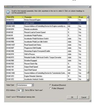
Two CAN interface ports are included, which allow connection of two independent CAN networks. CANgate's versatile configuration options allow you to select the parameters of interest, apply statistical functions (average, minimum, maximum) and control the format in which data are returned. CANgate supports widely used protocols such as ISO-15765 and SAE-J1939, as well as raw CAN frames.
