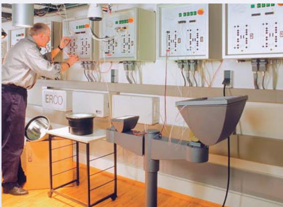
Thermal testing of luminares in a testing laboratory
