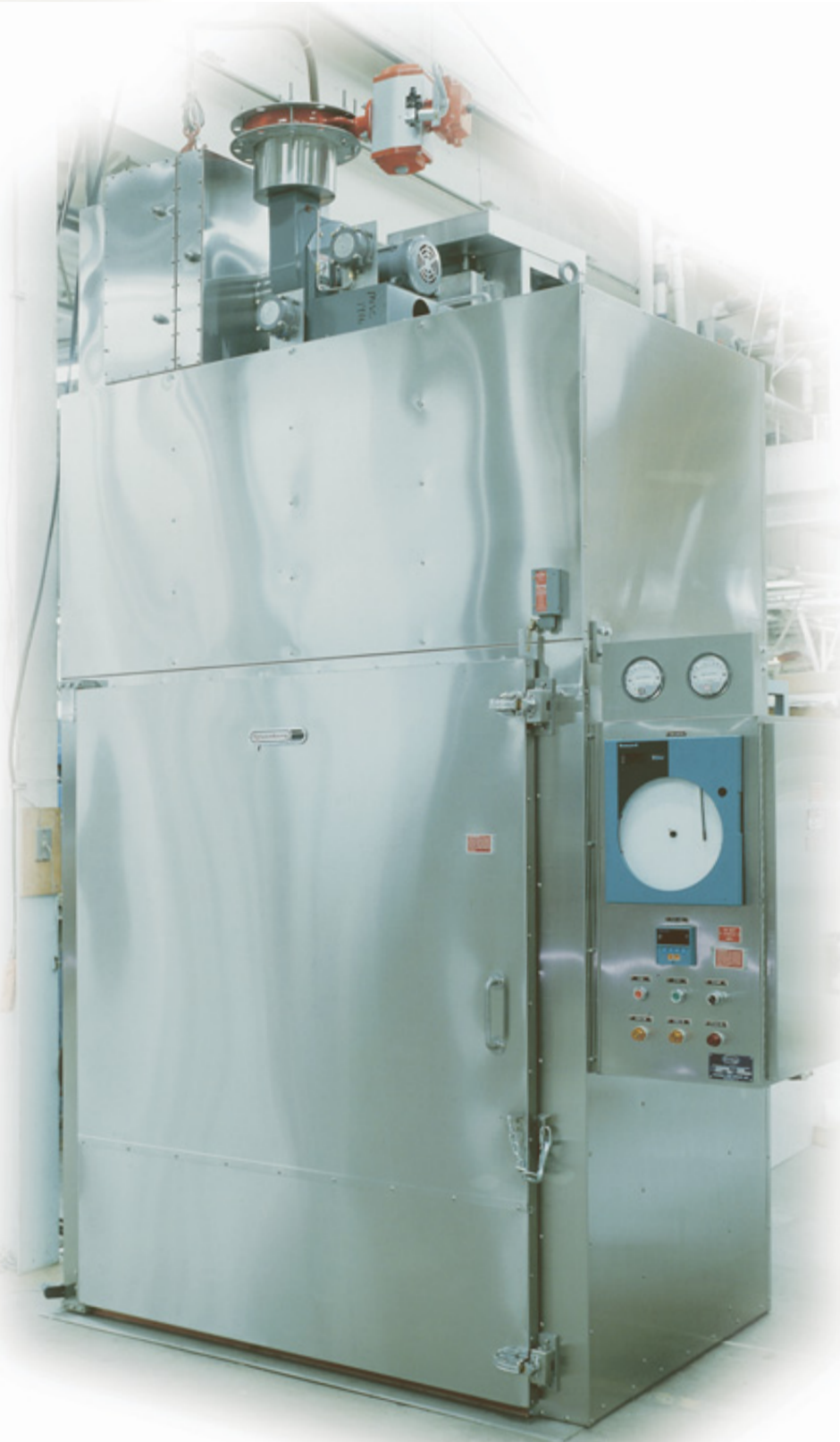
A custom-built device to supply conditioning air to a remote chamber. Class I, Division I Class.
